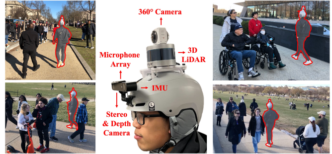
Fig. 1: Data collection in natural human-inhabited public spaces with the open-source sensor suite including 3D LiDAR, stereo and depth camera, IMU, microphone array, and 360° camera.
