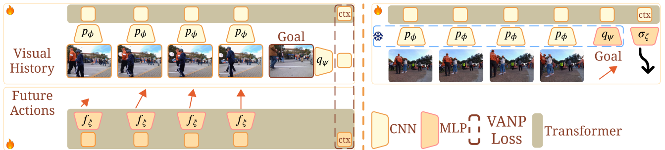
Fig. 2: VANP Architecture. VANP learns to embed temporal features into spatial features by using a sequence of images and leveraging two TransformerEncoders with context tokens. VANP’s loss maximizes the mutual information between history, future actions, and the goal (left). Then, by appending an MLP to the Transformer context token, VANP predicts future trajectories during the downstream navigation task (right).
